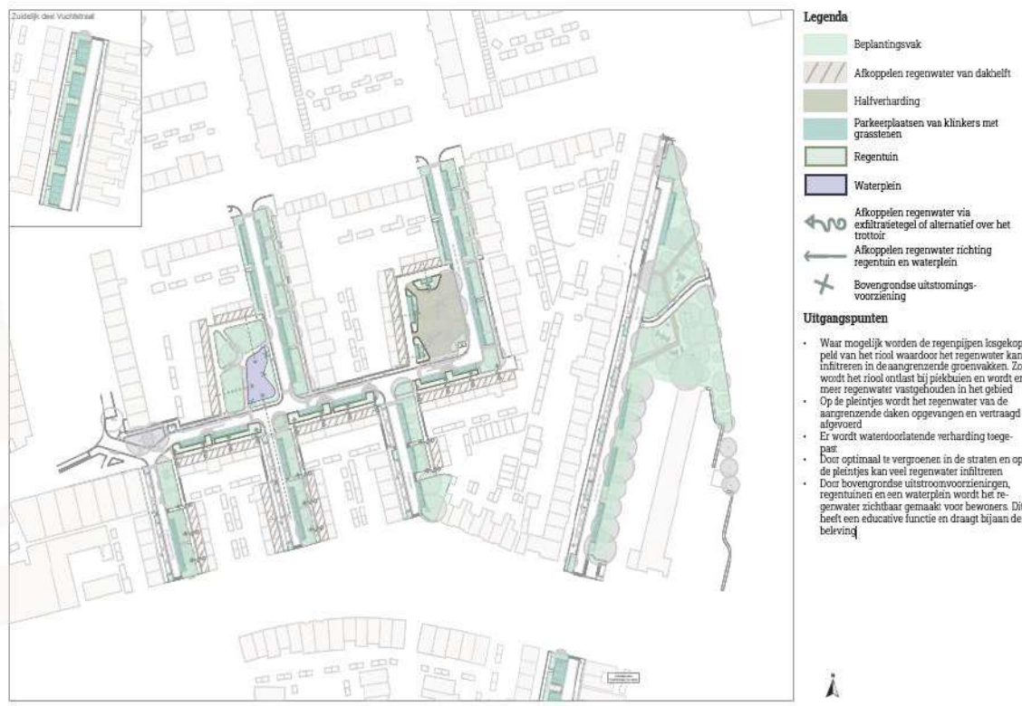
Figure 7.3.6: Adjustment to design elements in the Breda site to include consideration for rainwater collection and infiltration
