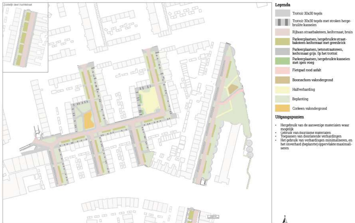
Fig. 7.3.5: Adjustment to design elements in the Breda site to include a consideration of materials
